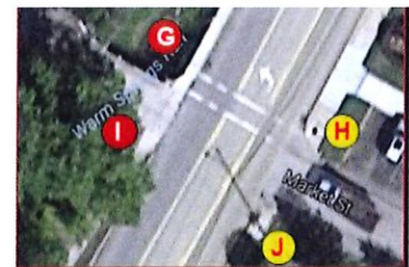
There is 1 marked crosswalk at this intersection. The existing ramps do not meet ADA dimensions and there are no DWS warnings
